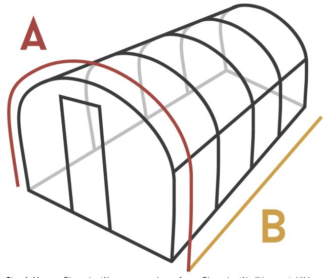
**Step 1:** Measure Dimension 'A' on your greenhouse frame. Dimension 'A' will be your 'width' measurement for your greenhouse or blackout material. This measurement should be taken using the full length of the support beam as pictured. We recommend adding 6 inches to 12 inches to this measurement to get a full edge to edge seal. Write this measurement down.
